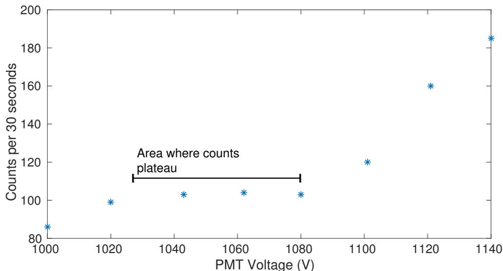
Figure 1. This plot shows the counts per 30 seconds versus different PMT voltages with the values for the detection threshold set at  $V_T = 0.092$  V. The middle of the plateau is at about  $V_{PMT} = 1060$  V. This data is used to find an appropriate  $V_{PMT}$  value for detecting muons.
